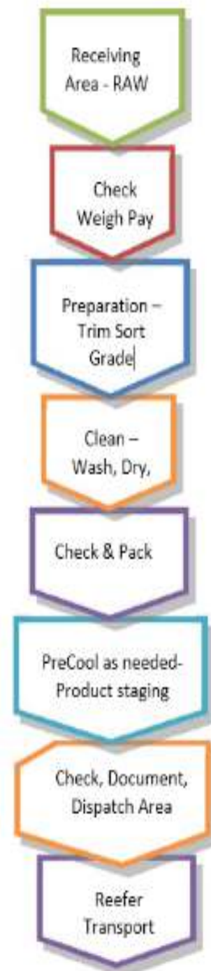
Flow chart for Step wise operations in Integrated pack Houses
